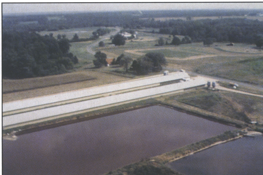
Wastewater from these poultry houses is treated in a lagoon system and then recycled as flush water. Excess is land applied.
