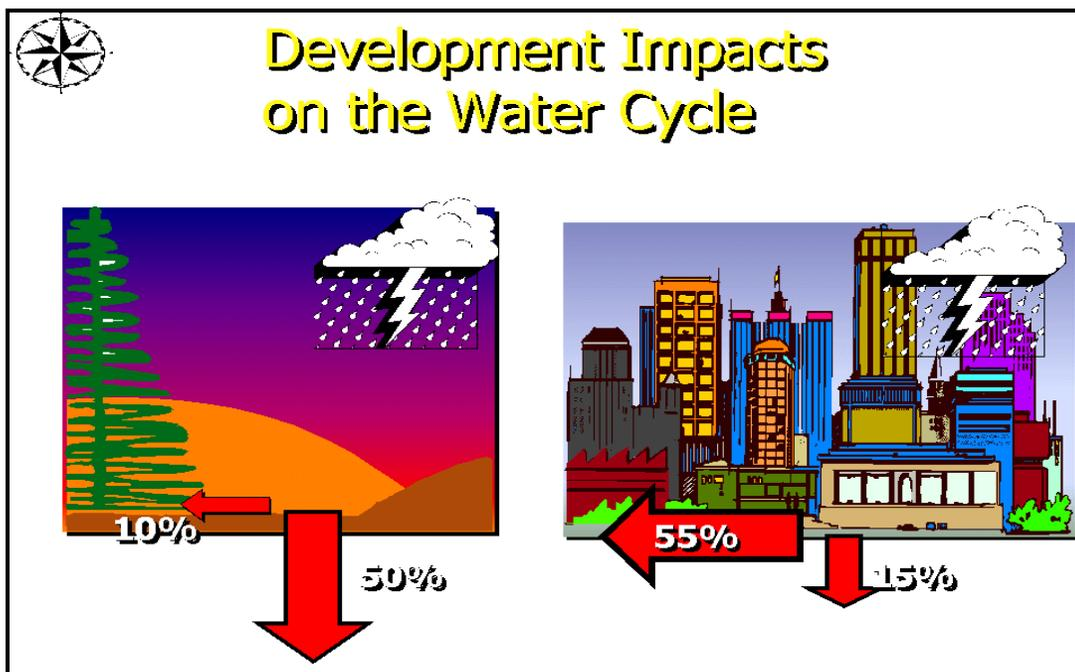
Infiltration of stormwater on an undisturbed landscape is around 50 percent, while stormwater runoff is around 10 percent. When a landscape is hardened by *impervious surfaces* such as roads, roofs, and parking lots, approximately 55 percent of stormwater is lost to runoff and only around 15 percent infiltrates.
