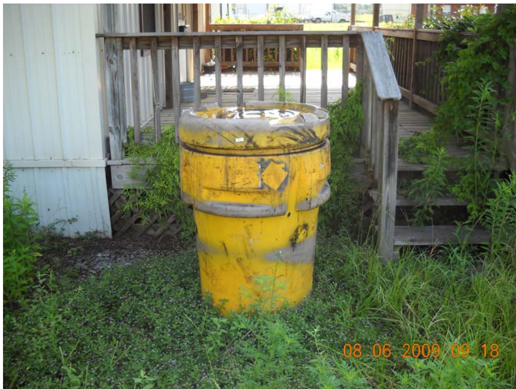
Over-packed drum containing waste paint
