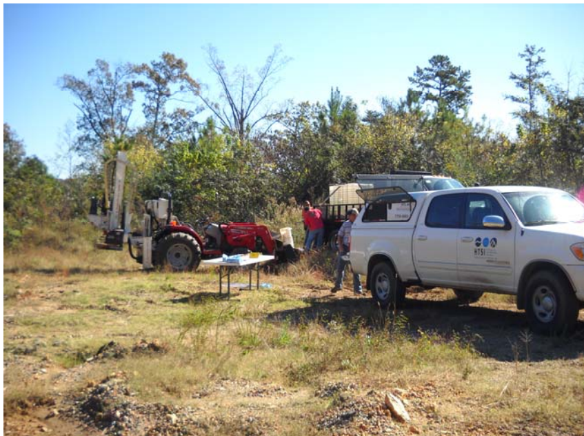
Environmental contractors collecting groundwater samples
