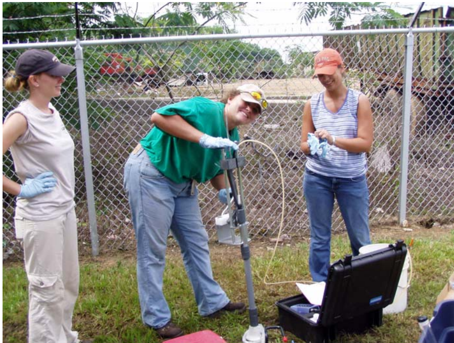
Groundwater Sampling at Temporary Monitoring Well #1 Montgomery Pilot Brownfield Site, Montgomery, Alabama
