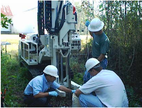
GeoProbe sampling performed at Prichard Brownfield site
