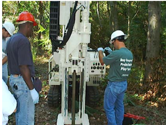
GeoProbe sampling performed at Prichard Brownfield site
