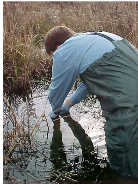
ADEM personnel performing surface water sampling at the Coliseum Boulevard Plume Site
