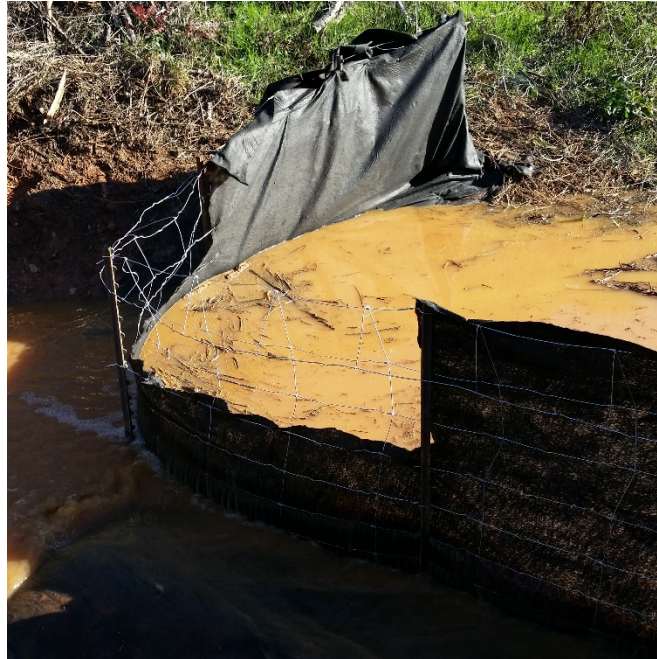
Figure CD-7 Silt Fence Check Dam (Photo courtesy of Auburn University Erosion and Sediment Control Test Facility)
