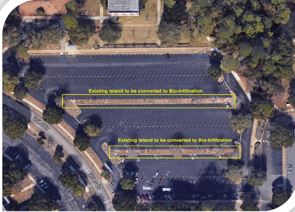
These are the locations for BMP practices for the placements of the bio-infiltration swales in the Humanities Parking lot (above), and a picture of the completed swales (on the right and below).
